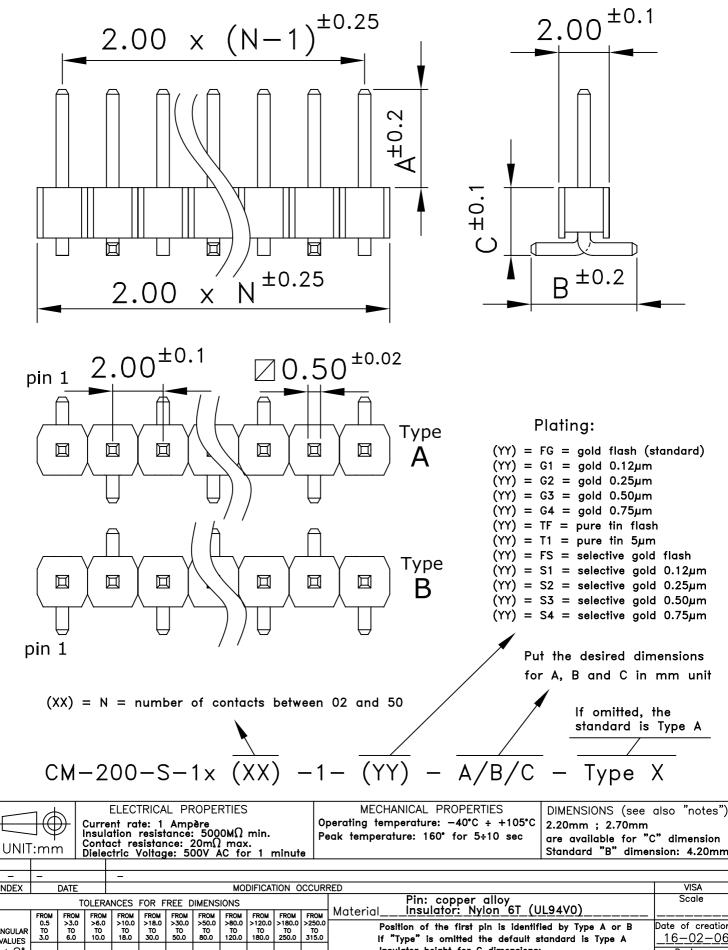
INDEX ANGULAR VALUES Insulator height for C dimensions: Designer  $\pm 2^{\circ}$ ±0.125 ±0.150 ±0.180 | ±0.215 | ±0.260 | ±0.310 | ±0.370 | ±0.435 | ±0.500 | ±0.575 | ±0.650 1.5mm when C is 2.2 and 2.0mm when C is 2.7 Notes: Part number: CM-200-S-1x (XX) -1- (YY) -A/B/C - Type X
